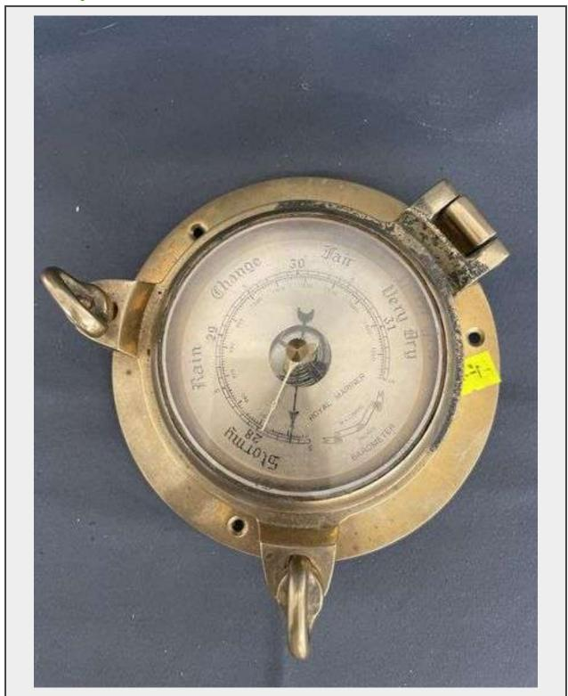
**Description**Royal Mariner barometer with a brass casing. Indicates weather conditions from Stormy to Very Dry.
